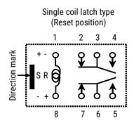
S: Coil polarity for Set R: Coil polarity for Reset
