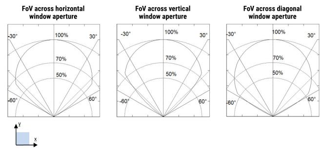
Note: Normalised polar plots show typical FoV along x, y axis and diagonal with 4.48 µm/620 nm filter applied, with infrared source being a blackbody radiator at 500 K temperature.
