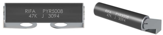
The PYR resistors are wire wound on a ceramic core and coated with high temperature silicone. The mounting brackets are made of stainless steel and connected by two point spot welding.
