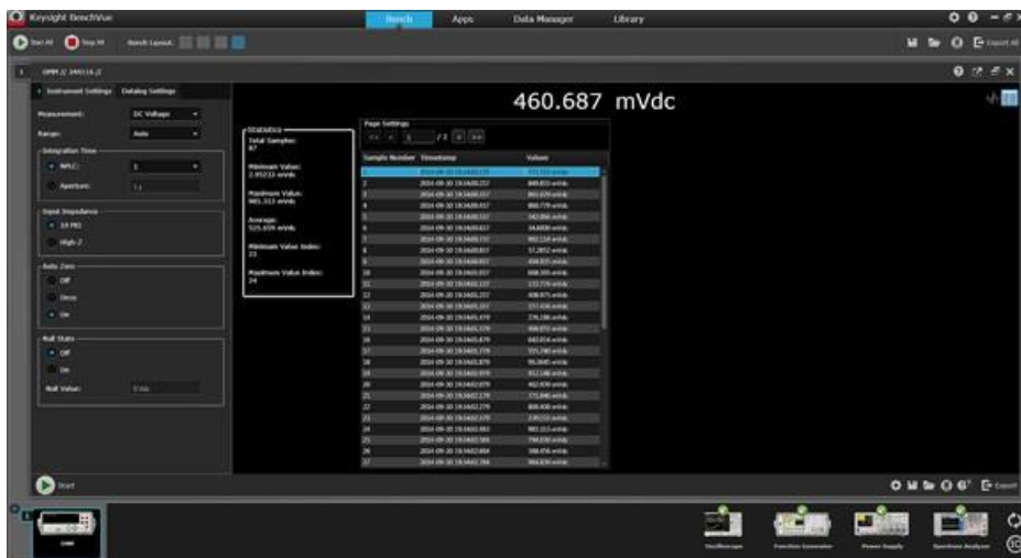
Figure 2. BenchVue enables control of your DMM to data log and visualizes measurements in a wide array of display options.
