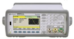
Control your function generator to set waveform properties and load custom arbitrary waveforms from files or drag-and-drop from an oscilloscope.
