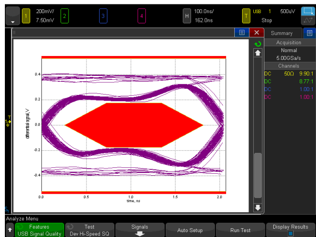
Figure 10. USB 2.0 signal quality eye test based on USB-IF physical layer compliance standards.
