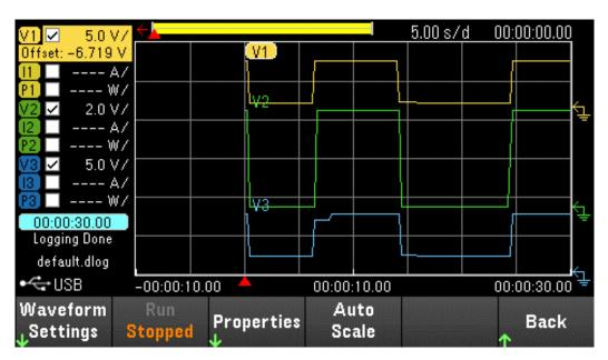
Figure 7. In Data Logger View, you can log data on multiple traces. Here the voltage of output 1, output 2 and output 3 are captured over 30 seconds
