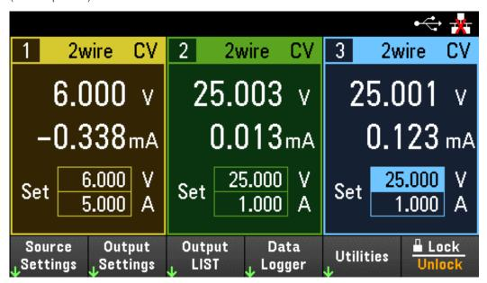
Figure 4. View all three outputs simultaneously.
