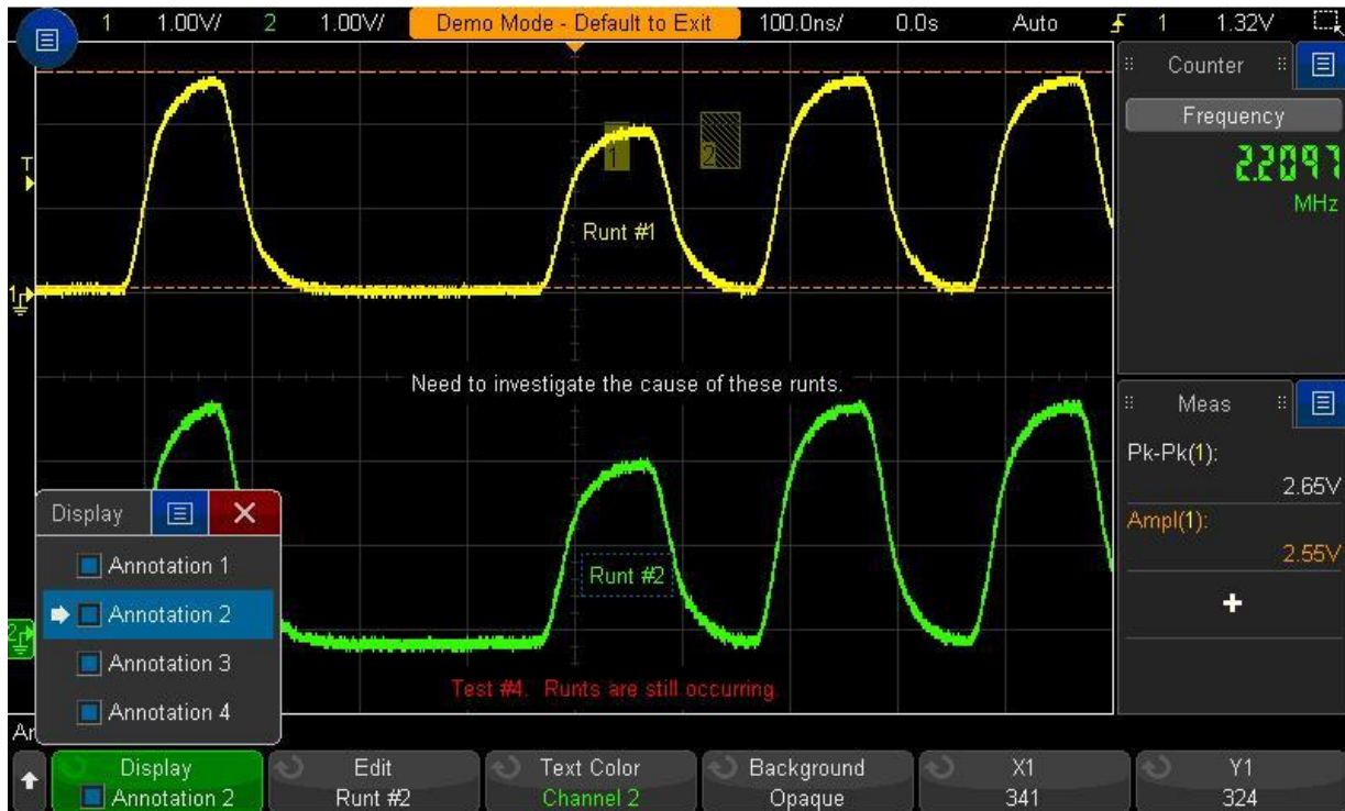
Figure 5. See up to ten annotations on screen at once for documentation. The standard touch screen makes inputting notes simple.
