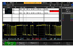
Figure 17. CAN-FD decode and trigger.
