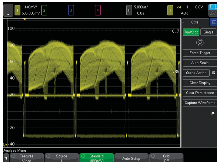
Figure 27. Triggering on 1080p HDTV signal analysis.
