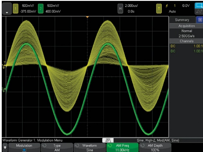
Figure 22. WaveGen sine wave output with and without added AM modulation.
