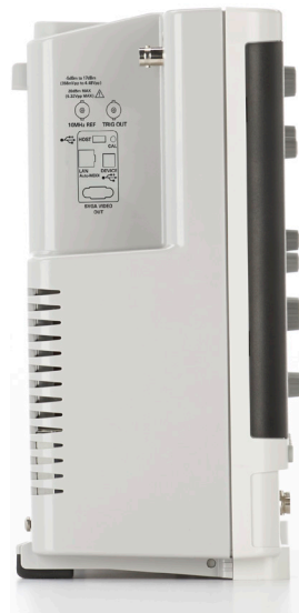
Figure 8. One-gigahertz-per-inch form factor: 6 GHz, 6 inches deep.
