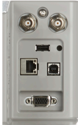
Figure 52. Connectivity section on the back panel.
