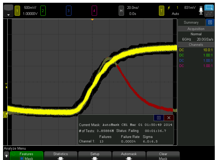
Figure 40. Limit testing of infrequent glitch.
