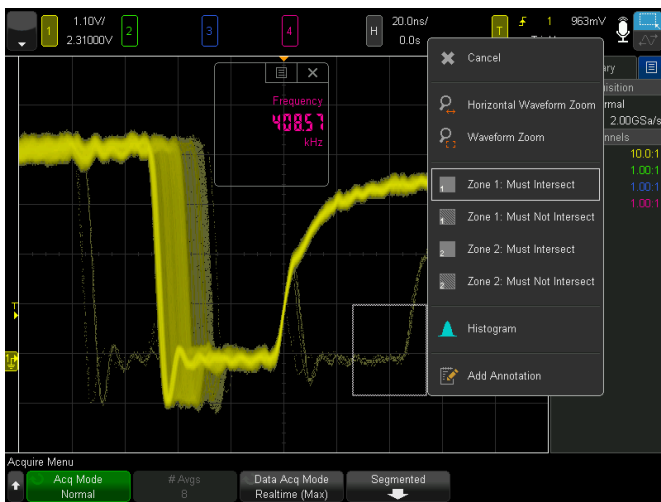
Figure 11. Draw a zone (box) around the anomaly.
