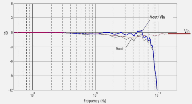
Swept frequency response with a 25- \Omega source
