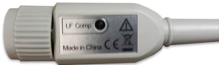
Figure 2. Low-frequency compensation adjustment (for N2840A/41A/42A/43A/53A)
