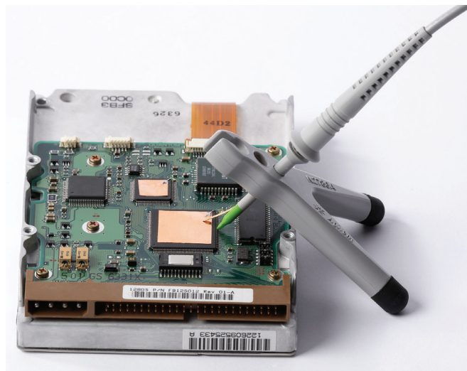
Figure 8. An IC cap adapter and ground blade with optional N2786A two-leg probe positioner offers an ideal hands-free solution for short circuit-proof probing of a fine-pitch IC. The N2877A deluxe accessory kit and N2878A fine-pitch accessory kit contain one N2786A two-leg probe positioner.
