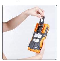
3) Press the stand down into its hinge.
