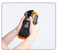
4) To disassemble, pull out the adapter.
