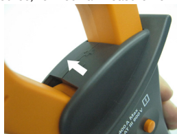
Figure 3: Conductor Alignment Direction
