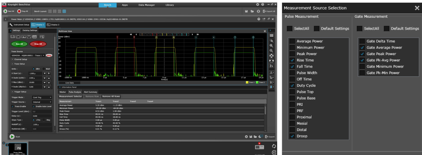
Figure 9. Multi-channel trace display with 4-pairs of gates and automatic pulse parameters measurement (sample screen shot with two U2042XA).
