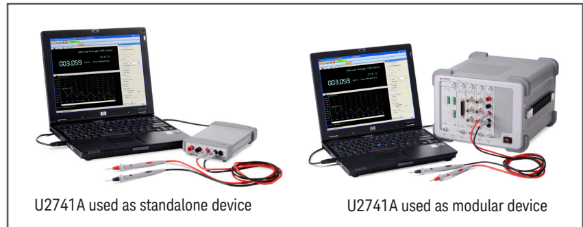
Figure 1. The U2741A DMM showing dual-play capability
