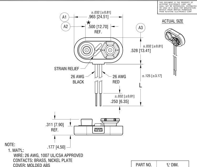
2. RED WIRE CONNECTED TO FEMALE CONTACT; BLACK WIRE CONNECTED TO MALE CONTACT.
