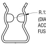
R.125 [R3.18] TYP. (DIAMETER TO ACCEPT 250 DIA. FUSE.)
