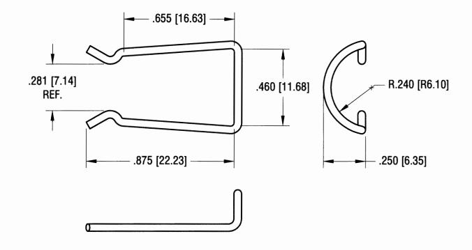
KEYSTONE ELECTRONICS CORP. ASTORIA, N.Y. 11105-2017 PART NAME BATTERY RETAINER CLIP, 'AA' MATERIAL .045 [1.14] DIA. STAINLESS STEEL FINISH BOONE 10.7.81 2.5X 9.26.05 CHANGE AS PER ECN 05-071 Α TOLERANCES INCH [MM] CODE DWG NO. DECIMAL ± .010 [± 0.25 ] ANGULAR ± 1° UNLESS OTHERWISE SPECIFIED 61 C DATE DESCRIPTION REV.
