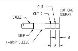
${\bf 1}$  . Cut the cable end square. Slide the k-grip sleeve onto the cable. Make "Cut 1" and "Cut 2" in the Jacket.
