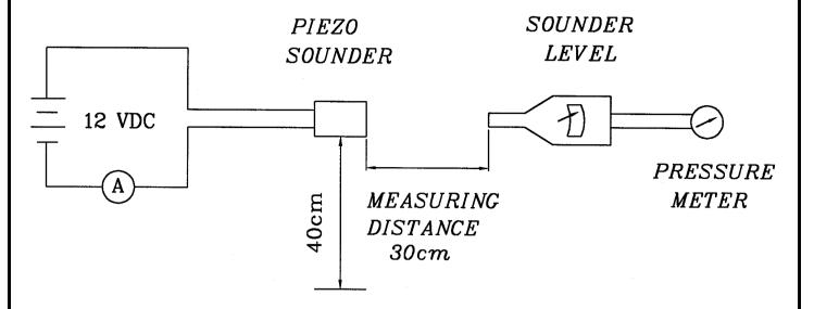
$\mbox{Mic}:\mbox{RION}$  S.P.L meter UC30 or equivalent
