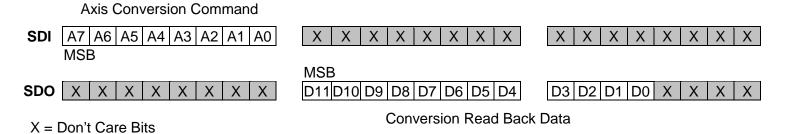
Figure 6 Register Diagram for 12-Bit ADC Read Operation
