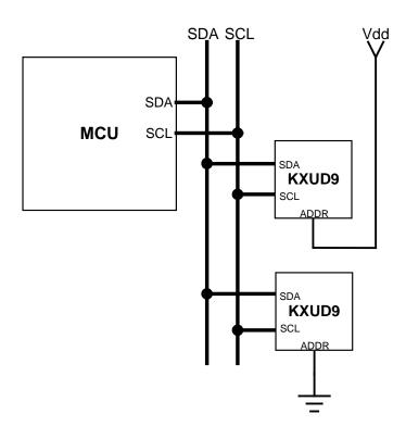
Figure 1 Multiple KXUD9 I<sup>2</sup>C Connection
