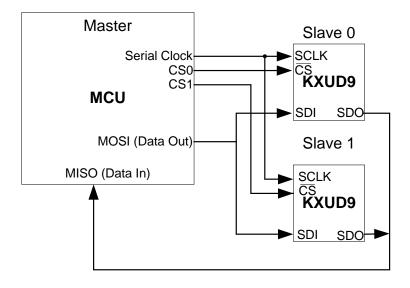
Figure 2 KXUD9 SPI Connections
