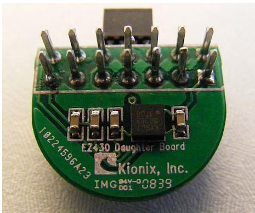
Figure 4: Kionix EZ430-7 Evaluation Board Mounted on TI eZ430-T2012
