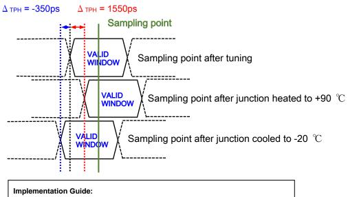
Host should design to avoid sampling errors that may be caused by the  $\Delta_{\text{TPH}}$  drift. It is recommended to perform tuning procedure while Device wakes up, after sleep. One simple way to overcome the  $\Delta_{\text{TPH}}$  drift is by reduction of operating frequency.
