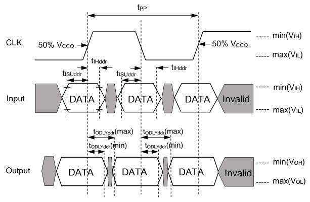
In DDR mode data on DAT[7:0] lines are sampled on both edges of the clock (not applicable for CMD line).
