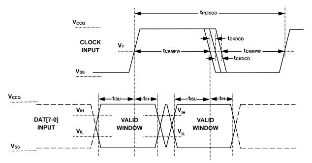
Note:  $V_T = 50\%$  of V<sub>CCQ</sub>, indicates clock reference point for timing measurements.
