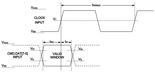
Note 1:  $t_{ISU}$  and  $t_{IH}$  are measured at  $V_{IL}$ (max.) and  $V_{IH}$ (min.). Note 2:  $V_{IH}$  denote  $V_{IH}$ (min.) and  $V_{IL}$  denotes  $V_{IL}$ (max.).
