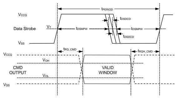
Note:  $V_T$  = 50% of V<sub>CCQ</sub>, indicates clock reference point for timing measurements.
