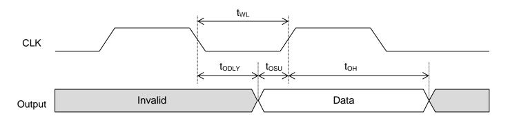
$t_{OSU}$  (min) =  $t_{WL}$ (min) -  $t_{ODLY}$ (max 8ns)
