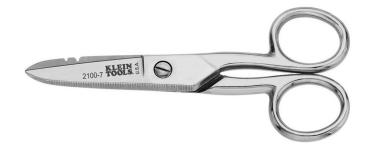
These Klein Tools Electrician's Scissors with stripping notches are made for telecom and electrical applications. They cut wire, cable and cordage including electrical communication 19 AWG and 23 AWG wire. The upper blade features wire stripping notches. The serrated lower blade allows for non-slip cutting action.
