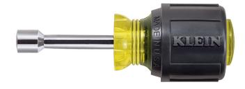
Full hollow shaft for work on stacked circuit boards or other long bolt applications. Allows for work in close quarters. Internal flanges provide solid, twist-resistant shaft anchor. Cushion-Grip handle allows for greater torque and comfort. Handle end is also color coded for easy identification.
