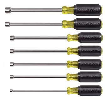
The Klein Tools Magnetic Nut Driver Set features nut drivers with internal flanges to provide a solid, twist-resistant shaft anchor. The nut drivers in this 7-piece set are made with chrome-plated, hollow shafts to help prevent corrosion. The donut-shaped magnetic tips easily hold fasteners in place for convenient use. The drivers are constructed with Cushion-Grip handles to provide greater torque and comfortable use.
