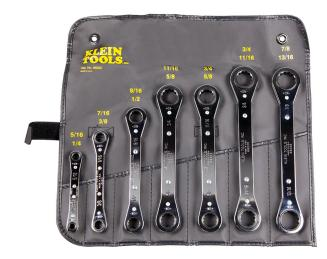
The Klein Tools 7-Piece Ratcheting Box Wrench Set contains a variety of standard wrenches for professional use. These wrenches are made from drop-forged steel alloy and are tempered for strength, light weight and long wear. These wrenches have a different size opening on each end for multiple applications.
