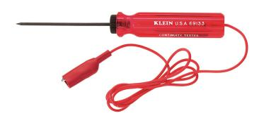
The Klein Tools Continuity Tester quickly reveals shorts or broken circuits in all types of electrical devices and controls. Tests for circuit continuity with power off. The pointed probes gets right to the problem. The handle lights up if the circuit is complete. Bulb for handle is included.
