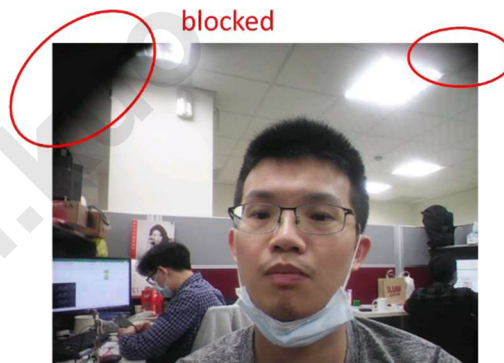
Figure 19: Image Corners are Blocked
