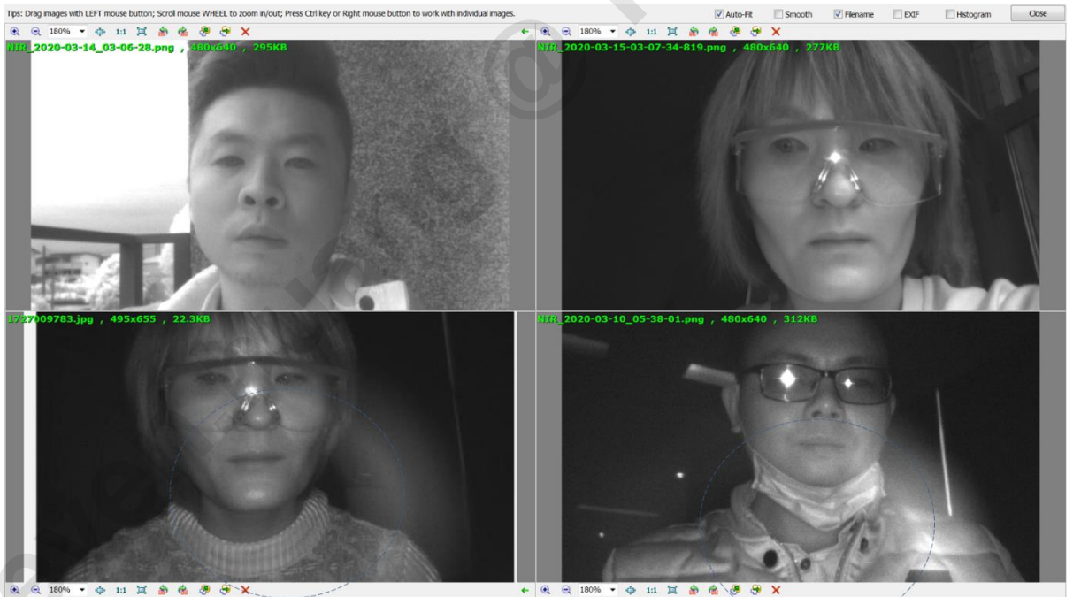
Figure – NIR images, we can see a ring if we turn on the LED
