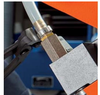
Sealing the hose connection on central lubrication
