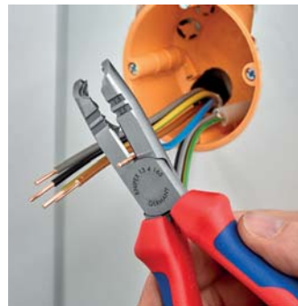
Cutting edges shortening of single wires
