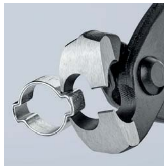
Using the side press nib
