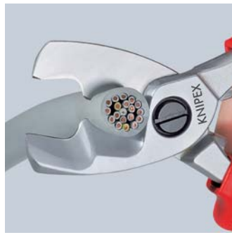
Final cut: after cutting the sheath in the front profile the conductors in the rear part are cut. Initial cut in the front profile, final cut in the rear profile – to keep it as easy as possible.
