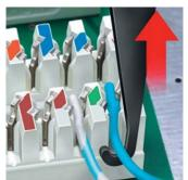
Putting down and cutting the cable in one
