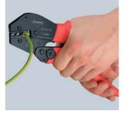
Third step: when greater hand force is required, such as e.g. when crimping insulated connectors 6 mm², two-hand operation is possible by the longer handles
