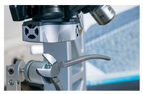
Shape and roughness of the diagonal cutter's cutting edge are precisely measured with an optical 3D measuring system.
