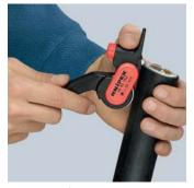
Setting the tool for longitudinal cut
