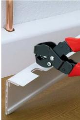
The KNIPEX Notching Pliers produces the most common notches in plastic ledges and cable ducts in a simple, fast and clean way. No time-consuming sawing out or nibbling and no additional work required.
