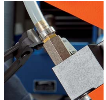
Sealing the hose connection on central lubrication
