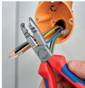
Cutting edges shortening of single wires
