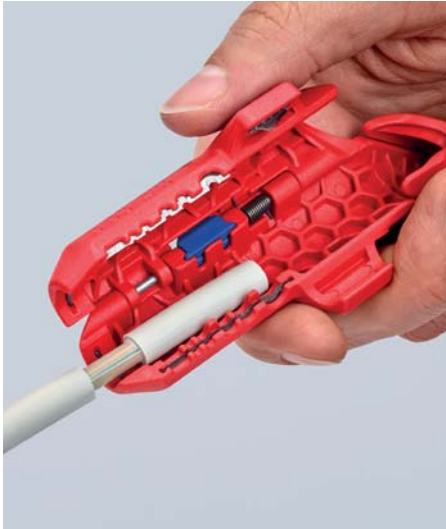
Dismantling of a NYM cable
