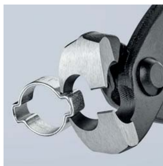
Using the side press nib
