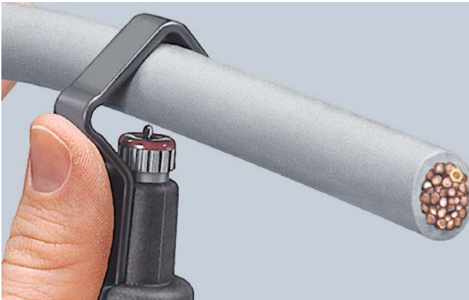
Setting the tool for circular cutting
