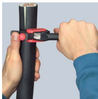
Turning the tool for circumferential cut
