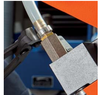
Sealing the hose connection on central lubrication
