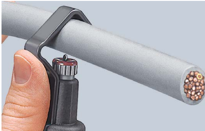
Setting the tool for circular cutting
