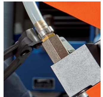
Sealing the hose connection on central lubrication
