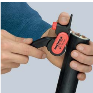
Setting the tool for longitudinal cut
