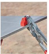
Plastic positioning jaw: tilting for a clean break line and optimum protection of the tiles against damage
