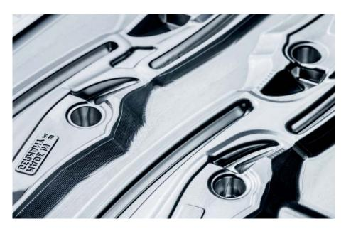
Forging die for the high leverage diagonal cutters with forged-in axle.
