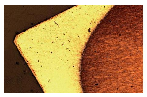
Macro image of a cutter after induction hardening. The specially hardened cutter area (light) is in sharp contrast to the softer structure of the body of the pliers (dark).
