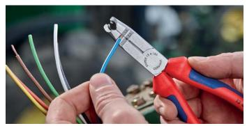
Stripping holes for conductors of 1.5 mm² and 2.5 mm²
