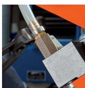
Sealing the hose connection on central lubrication
