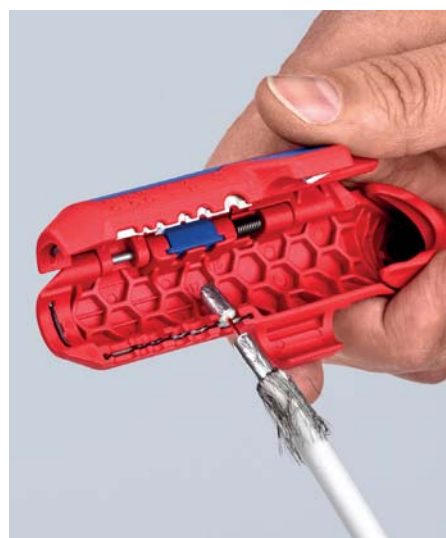
Stripping of a coax cable
