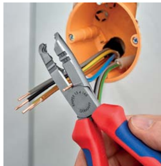
Cutting edges shortening of single wires
