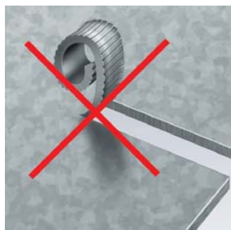
Notching without chip breaking
